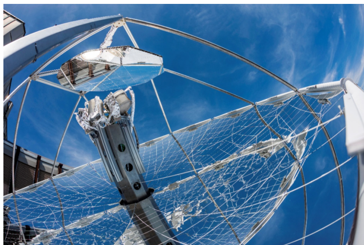
Figure 7.1.2: Solar refinery for converting CO 2 into fuel and oxygen, ETHZ
